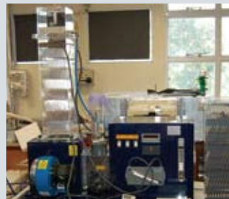
A mini-cooling tower in Building Services Engineering Laboratory.
