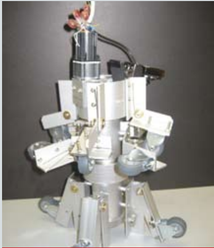
To extend the service life of underground pipelines, a unique robotic device was developed by a student project group to travel inside a gas pipe for spraying protective coating on its inner surface.
