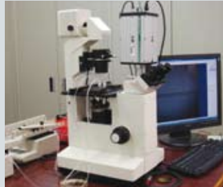
Equipment for studying flows in micro-channels which are, typically, few tens of \mu\text{m} in width.
