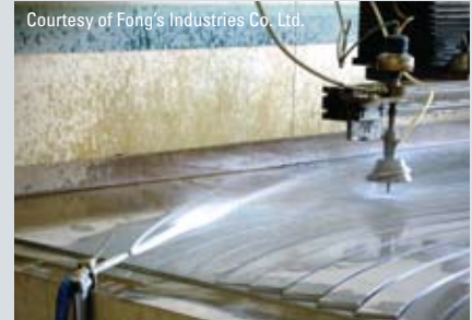
In waterjet cutting, a mixture of water and abrasive substance under high pressure are employed. It is the preferred method when the material being cut is sensitive to the high temperature generated by other machining method.
