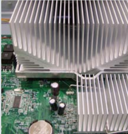
Heat sinks used in PC dissipate heat efficiently by using a large surface area to volume ratio.
