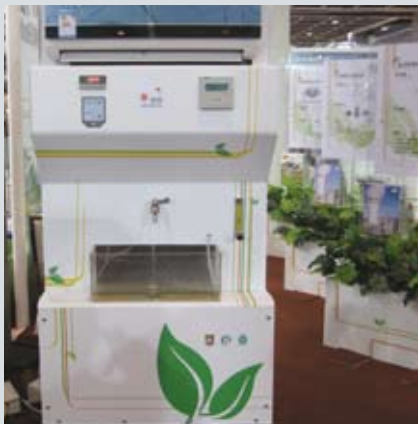
In large hotels, heat pumps are installed to extract the heat dissipated by air-conditioning systems to warm up tap water for sanitary use. The photo shows a small heat pump designed by our department under the sponsorship of Environment & Conservation Fund and Woo Wheelock Green Fund. The heat pump can be adopted in residential flats in which split-unit air-conditioners are used.
