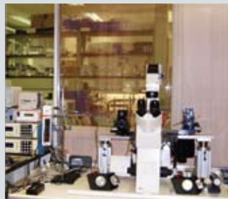
Micromanipulators for loading minute biotissues such as a living cell.
