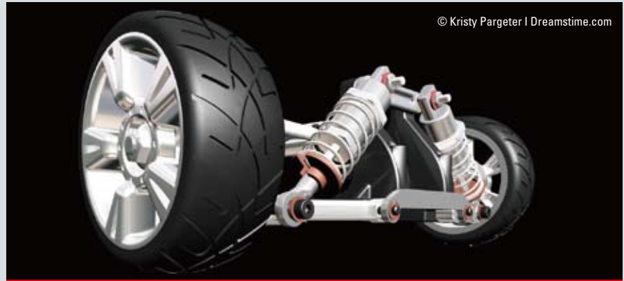
Springs and hydraulic dampers are commonly used in the suspension system of road vehicles.
