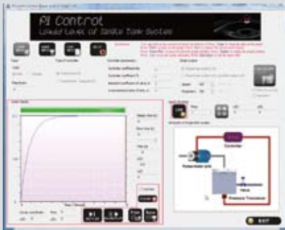
The output page of a computer project on simulation of liquid level controller.
